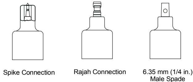
Figure 9: High Voltage Cable Connectors
